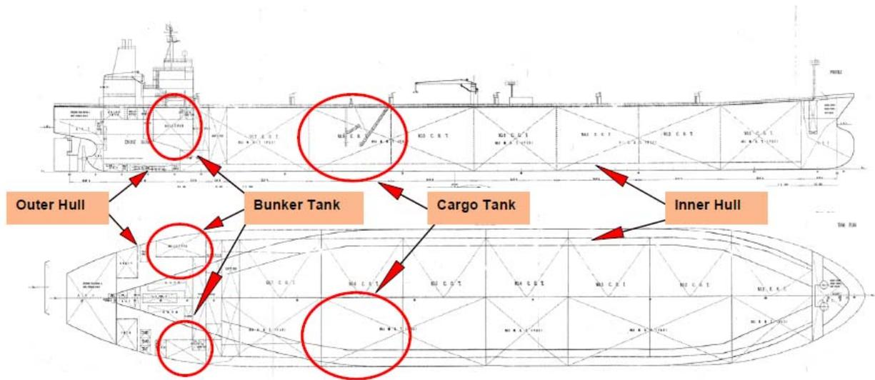
**Figure 2-3 General arrangement of a typical double hull tank ship**
