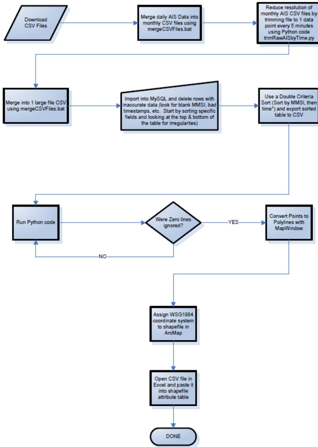
**Figure 2-2 AIS Data Manipulation Process**
